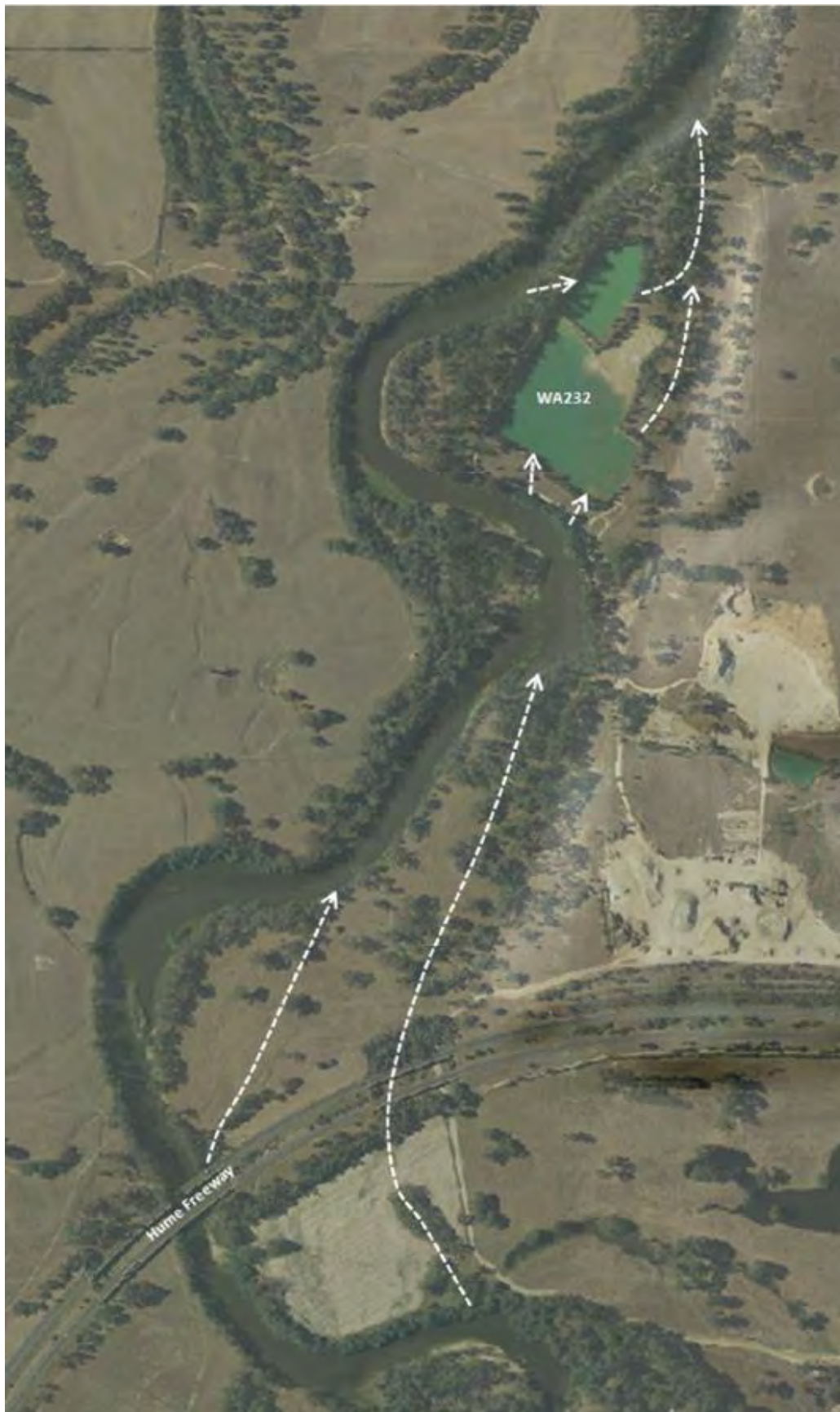
Potential avulsion paths and points of flow entry and exit into WA232 pit.
