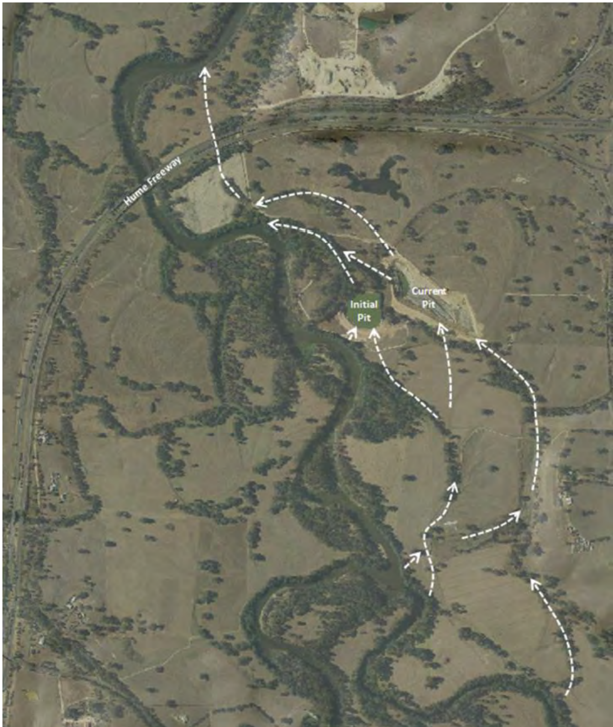
Preferred flow and potential avulsion paths and points of flow entry and exit into two pits at WA781.
