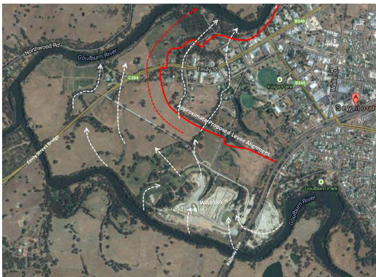
Figure 3.8: Preferred flow and potential avulsion paths and points of flow entry and exit into pit at WA1189. The approximate proposed levee alignment is also shown.
